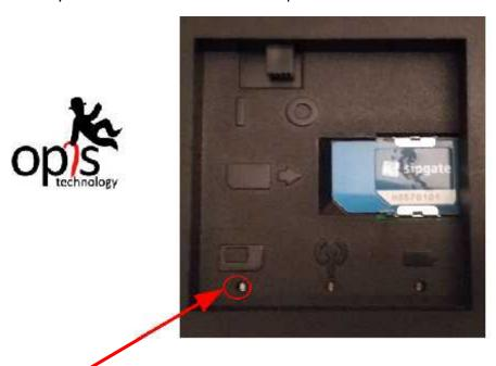
This LED should be off shortly after turning the phone on. In case it is not off is it:
